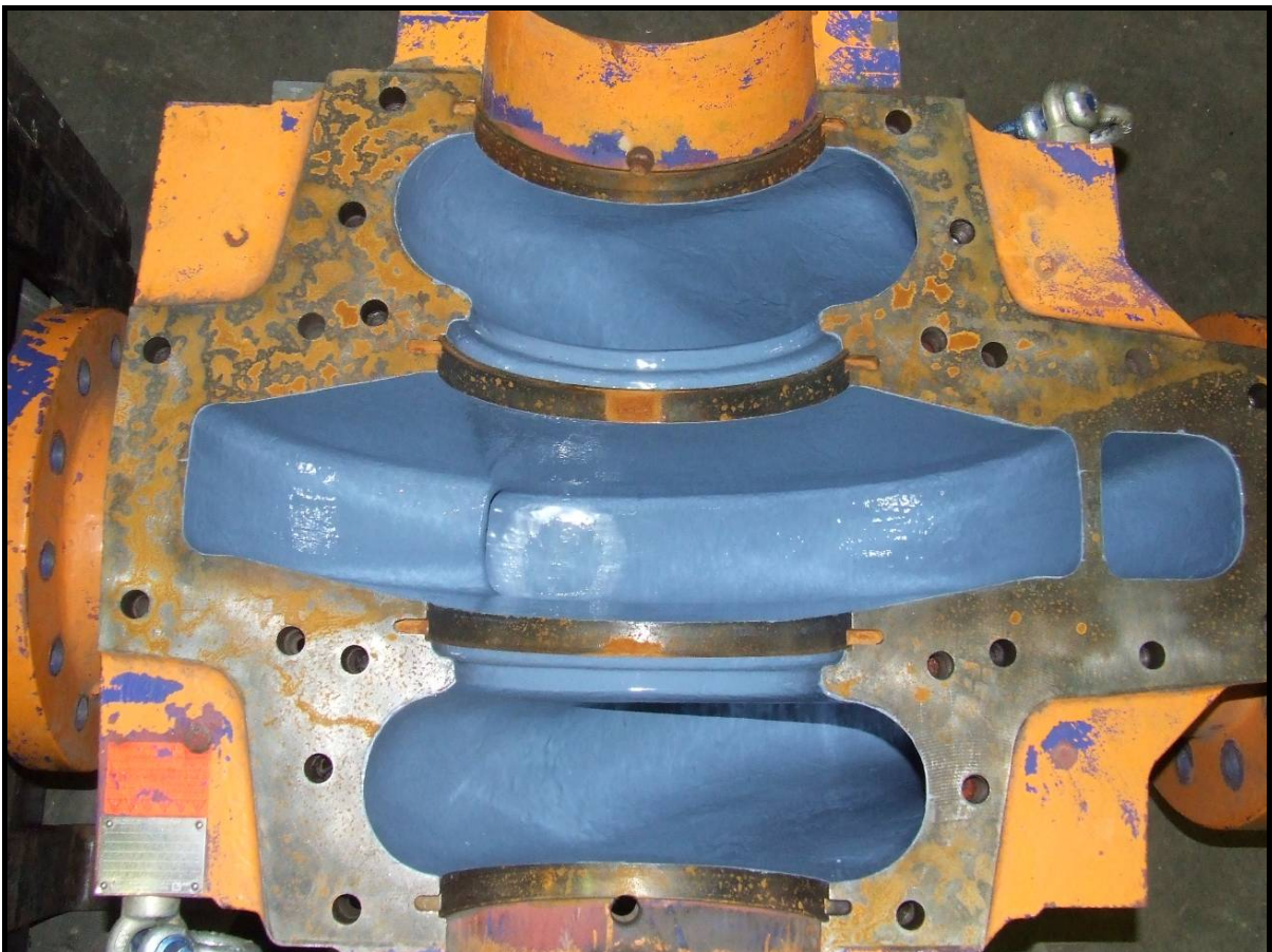
Picture 10 – Final surface finish – Pump casing
