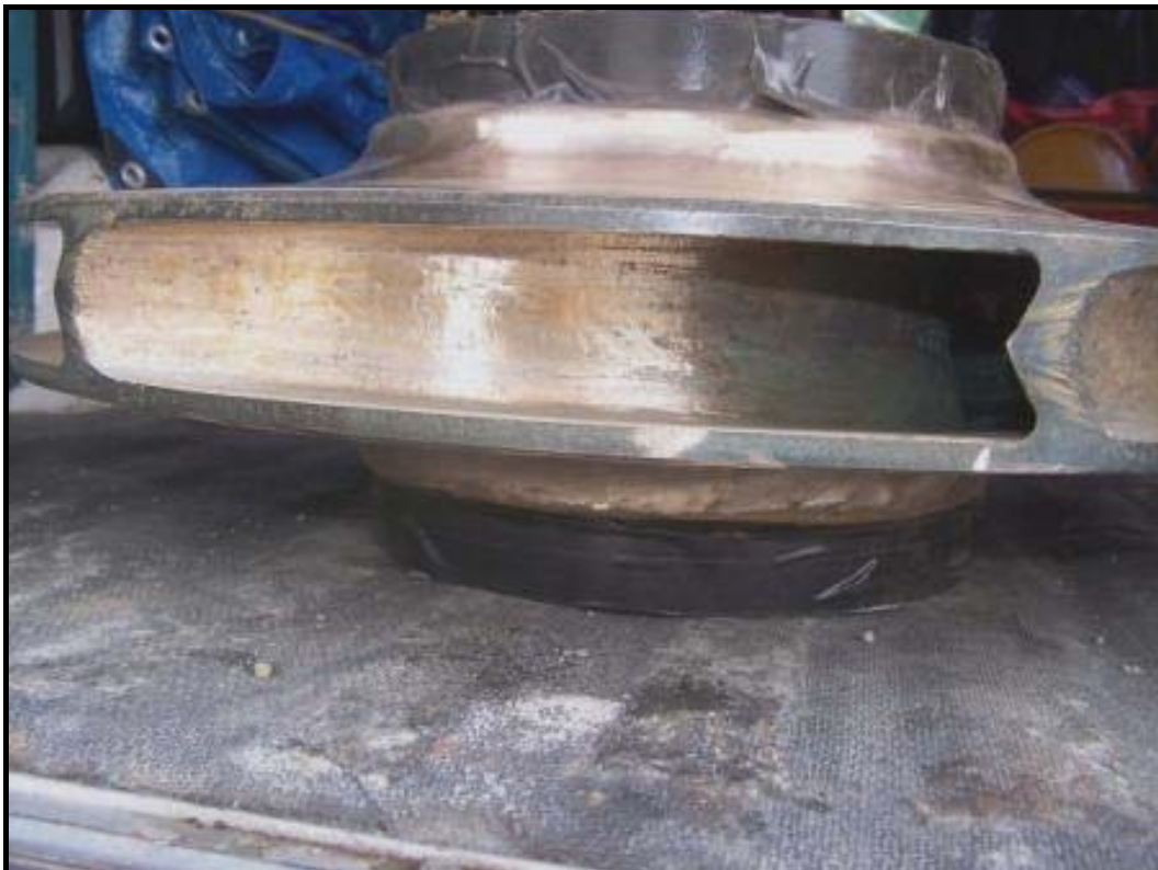
Picture 12 – Casting imperfection in pump rotor
